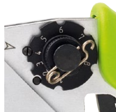
Crimp mandrel can be adjusted via Selector with 8 positions
