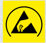
ESD Protective Symbol (for items that possess at least one ESD control property)
