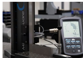
Checking the sides of bevel edge squares using the cylindrical measuring probe (optional) for GT31, since the measuring face is larger than with a ball-shaped measuring probe.
