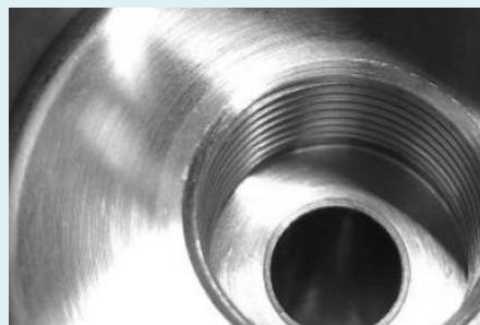
Turning contour and thread with boring bar stabiliser.
