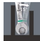
The small working arc of the open jaws is particularly suitable where space is tight.
