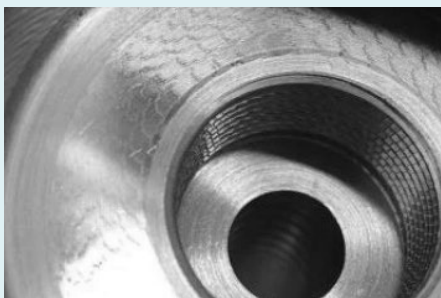
Turning contour and thread without boring bar stabiliser.
